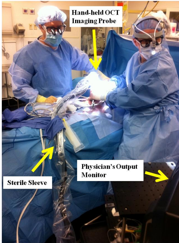
Figure 33. Intra-operative OCT/DOCT imaging of kidney post-reperfusion. The imaging system is kept several feet away from the operating table and only the handheld probe draped with a sterile sleeve is permitted to come into contact with bed and the patient.
